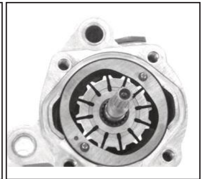
Install rotor dots down
