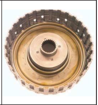
Remove forward clutch balance piston
