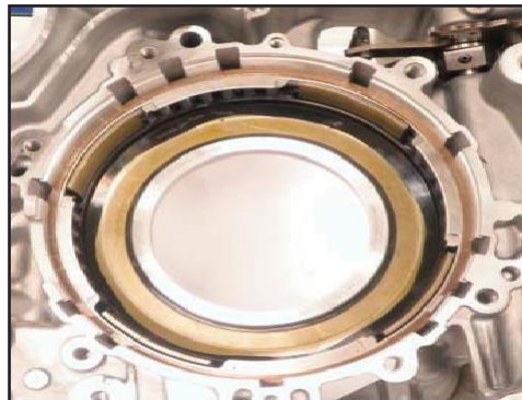
Remove reverse clutch, reverse clutch retainer and piston
