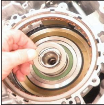
Install torrington bearing and planet carrier
