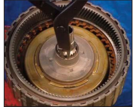
Install input shaft and snap ring
