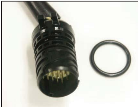
Install case connector into case
