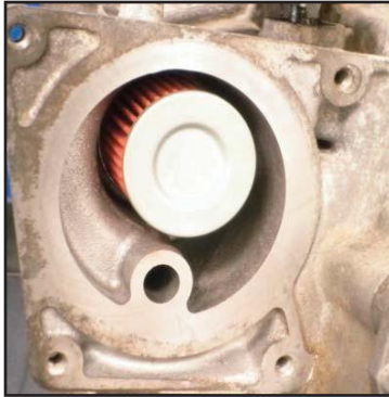
Install cooler filter
