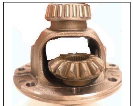
Remove both side gears and washers
