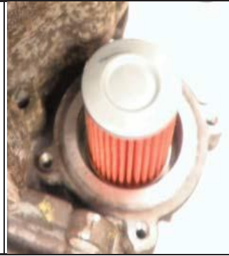
Install cooler filter
