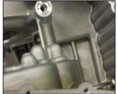
Tang on case connector faces down towards recessed in case
