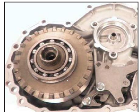
Remove the drive pulley
