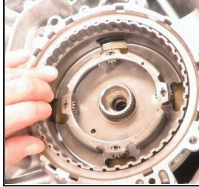
Install torrington bearing and planet carrier
