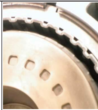
Install forward drum, drum is fully seated top of drum even with carrier
