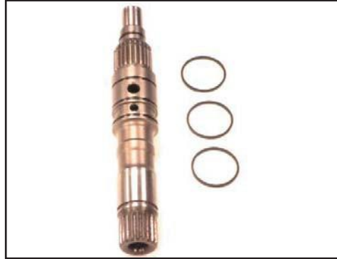
Replace input shaft sealing rings
