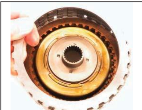
Install forward clutch pressure plate.
