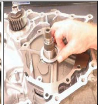
Install stator support and thrust washer
