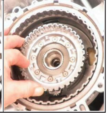
Install torrington bearing and sun gear into planet carrier
