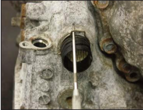
Remove clip holding in case center
