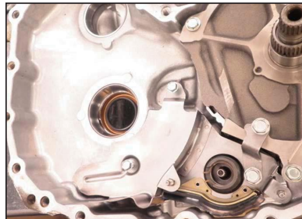
Remove the pump bracket to lower baffle and lower baffle.
