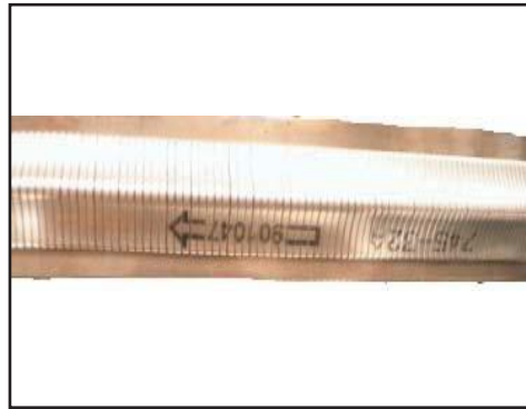
Install drive belt with arrow pointing to the left.
