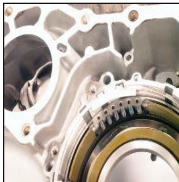
Compress retainer install snap ring
