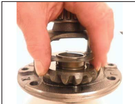
Remove both side gears and washers
