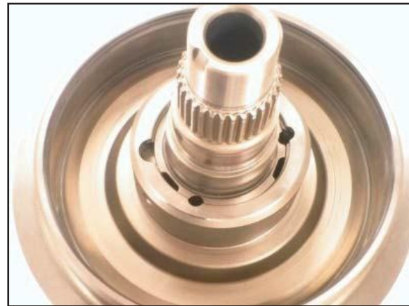
Remove piston retainer snap ring
