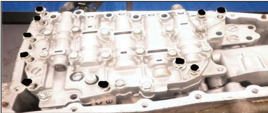
Remove marked bolts to remove valve body.
