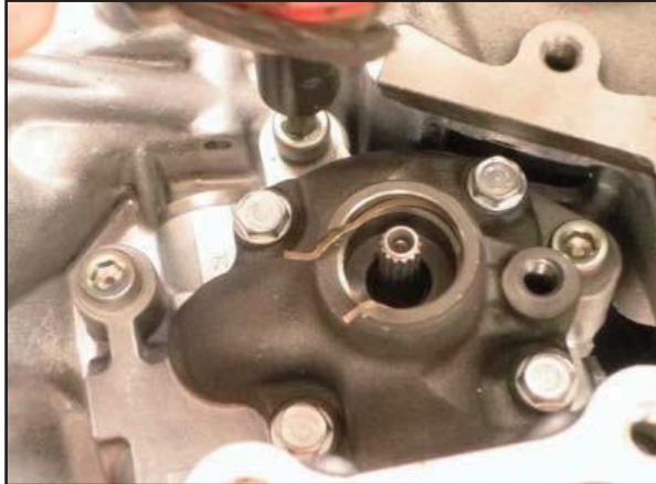
Remove the pump. There is one external bolt.
