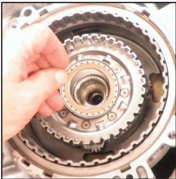
Install torrington bearing
