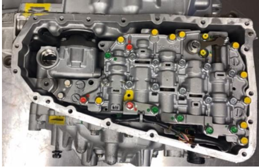
Install valve body and filter bracket
