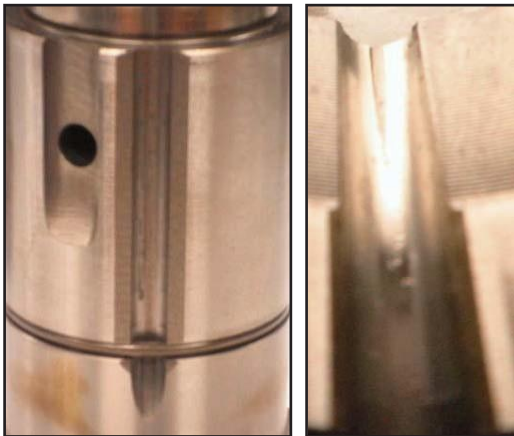
Compress balance piston
