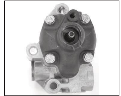
Torque cover bolts 19 Ft. Lbs. (26Nm)
