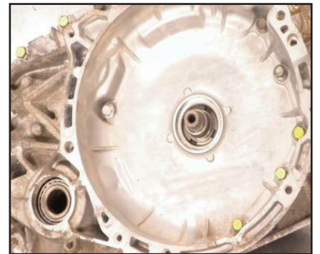
Using loctite 509 sealer, install the bell housing bolts marked in yellow. Torque to 33 Ft. Lbs. (45Nm). Bolts marked in yellow 1.67 in(42.8mm)
