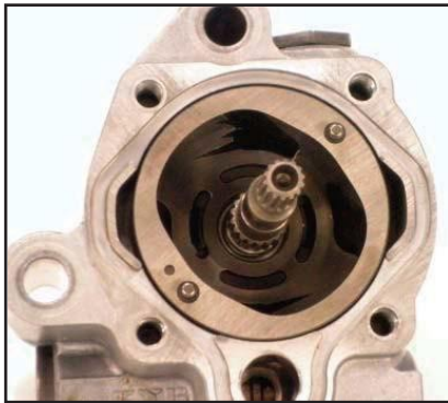
Install pump shaft
