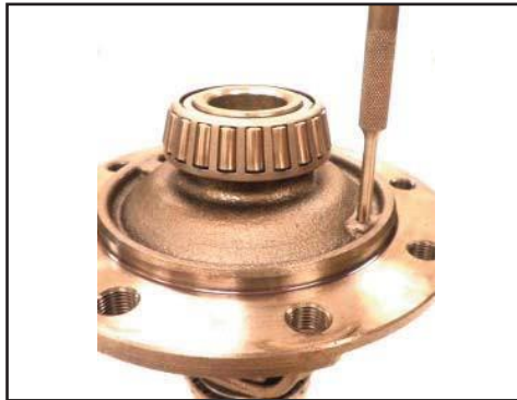
Remove differential roll pin
