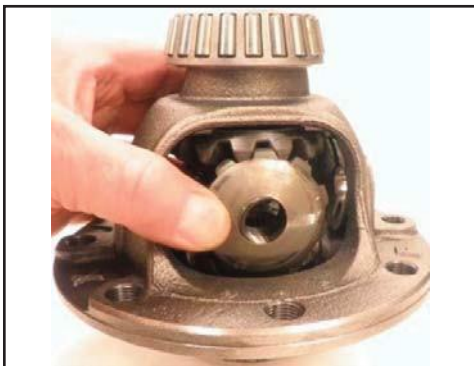
Rotate the spider gears 90° then remove the gears and the washers
