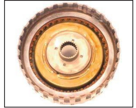
Install ring gear and snap ring
