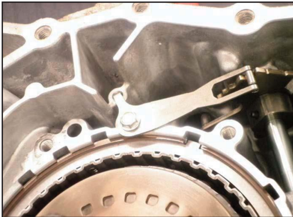
Remove detent spring
