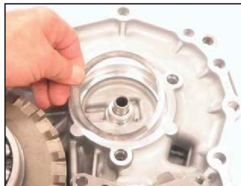
Remove the driven pulley shim
