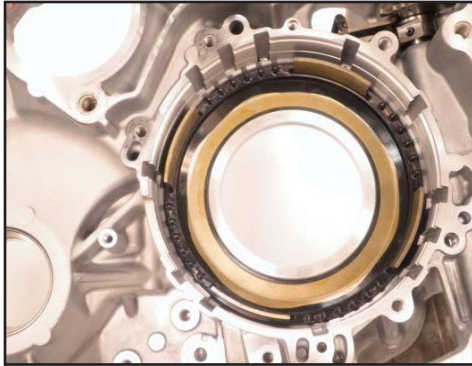
Install reverse clutch piston
