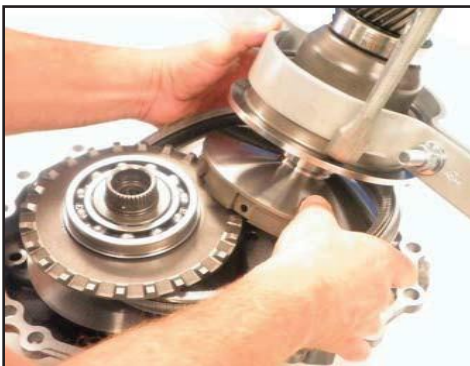
Remove driven pulley
