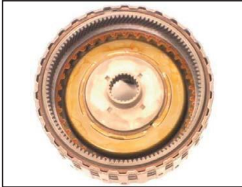
Install ring gear and upper snap ring
