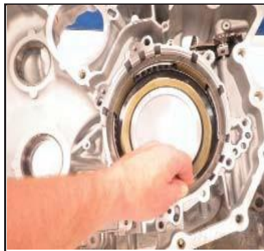
Install cushion plate, dish up
