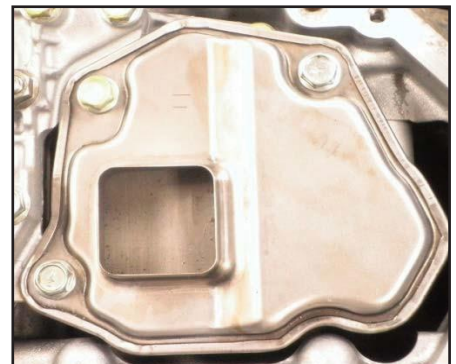
Install filter with new o-ring. Tighten bolts to 70 In. Lbs. (8Nm)
