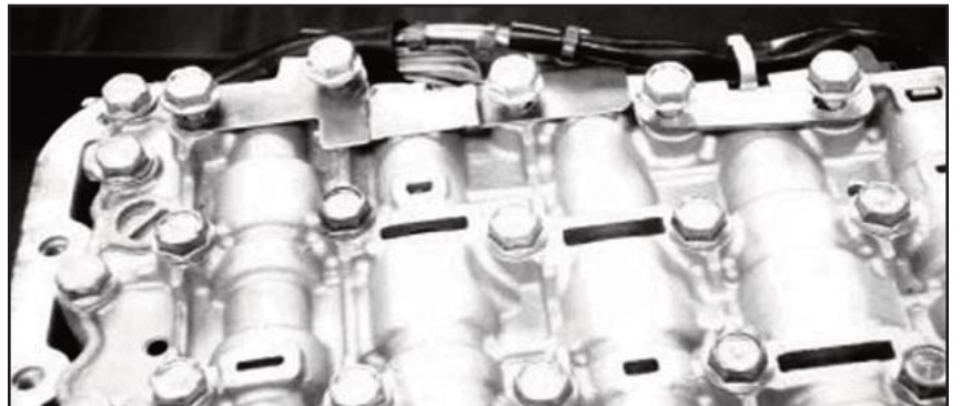
Remove the wire harness ROM (Read Only Memory Module)
