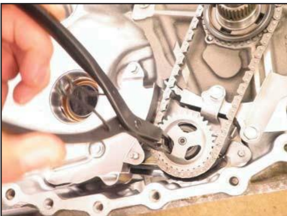
Remove pump driven gear chain and drive gear
