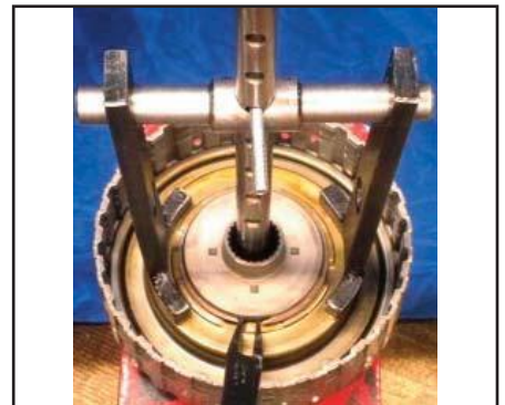
Install piston retainer/springs and snap rings
