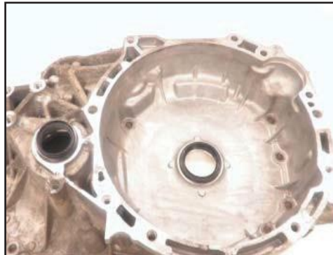
Install axle seal and front seal
