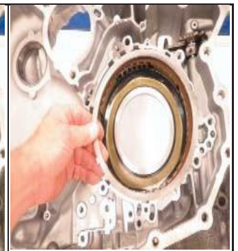
Install steel plate then friction plate, alternating ending with friction plate.
