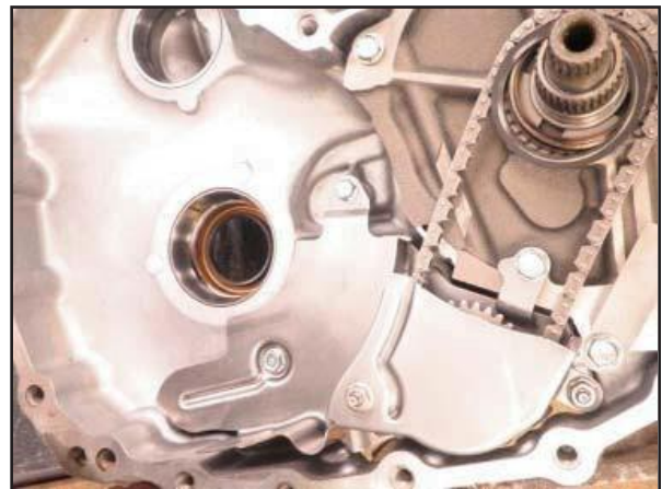
Remove o-ring, selective washer and upper baffle
