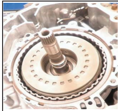
Install forward drum, drum is fully seated top of drum even with carrier
