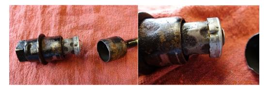
As you can see from the pictures this filter can be full of metal. The filter does have a bypass spring but if the filter is clogged it will cut down the cooler flow and it could cause overheating.
