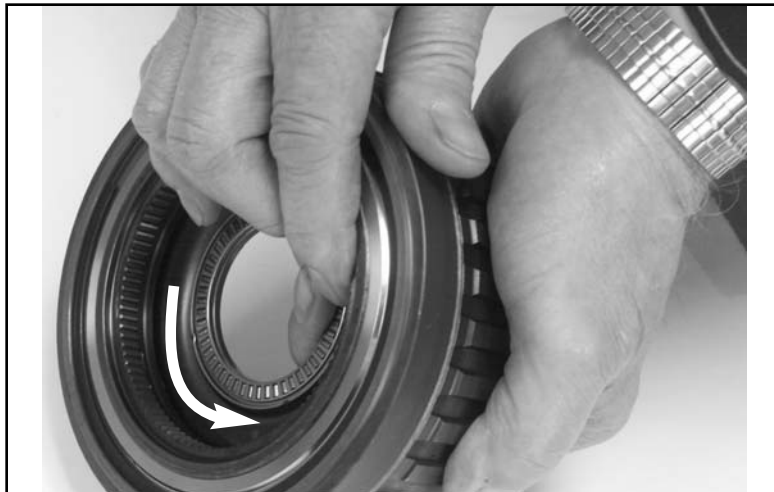
Inner race freewheels in counter-clockwise direction.
