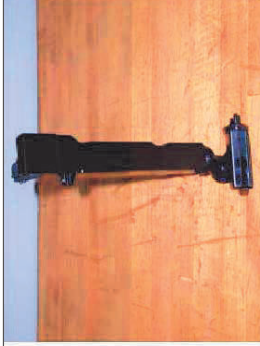
Fluid Level Control Valve (Outside Transmission)
