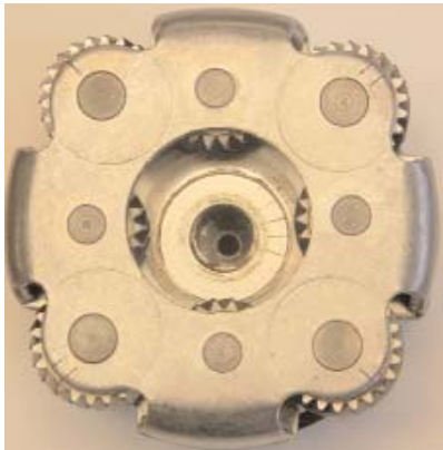
Align Timing Marks on 2:86 First Gear Ratio Planetary
