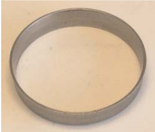
1-2 Servo Sealing Ring Compressor. Kent Moore Tool # J-38428
