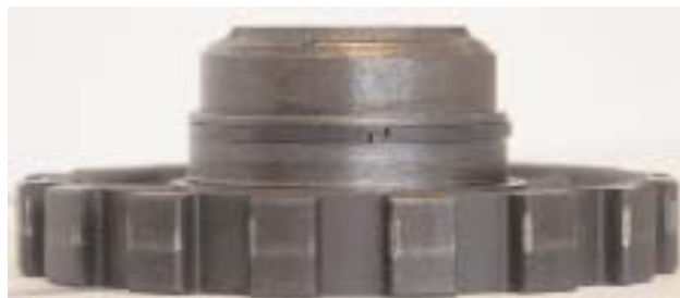
Sealing Ring on Parking Gear
