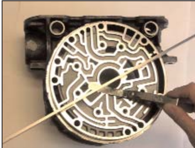
Checking Adapter Case for Warpage max Deflection .0015-.002
