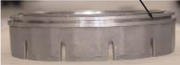
Two Different Overdrive Clutch Apply Pistons and Seals
