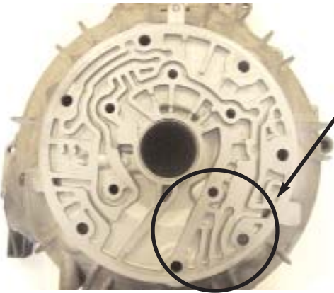
On/Off Torque Converter Clutch Bell Housing
