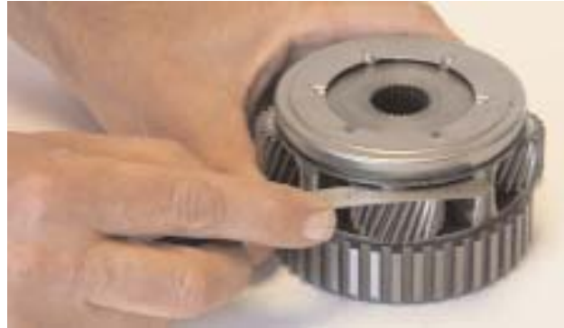
Checking Overdrive Planet Pinion Endplay. Clearance should be .009 - .025
