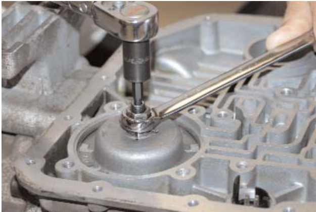
To adjust 1-2 band tighten servo adjusting screw to 40 inch pounds and back off 5 turns
