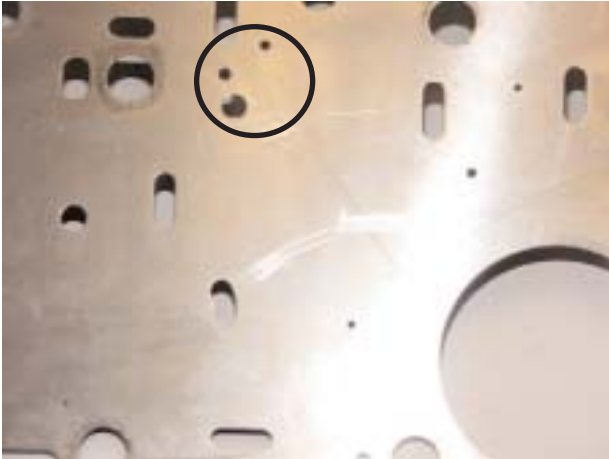
Type 1 Valve Body Plate Must Match Case
