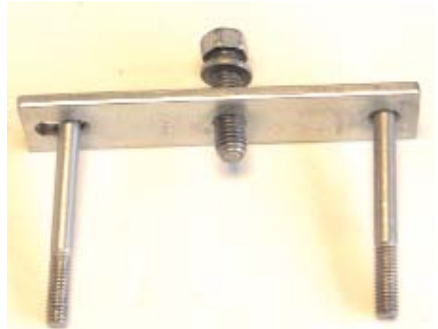
1-2 Servo Spring Compressor Tool made from Saver Bar
