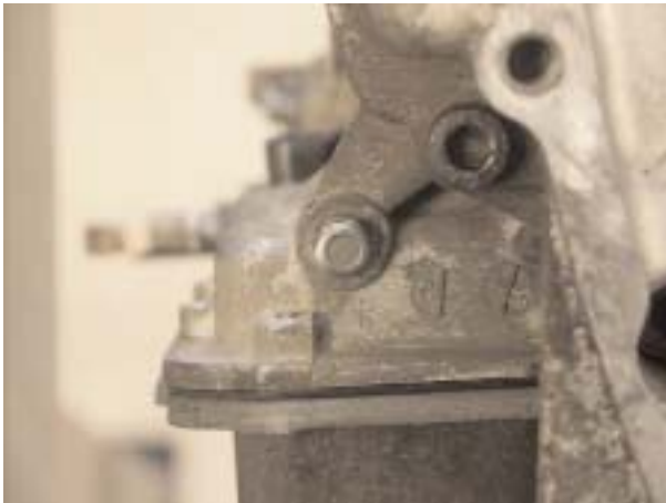
Drilled Case to Check Servo Release Pressure
