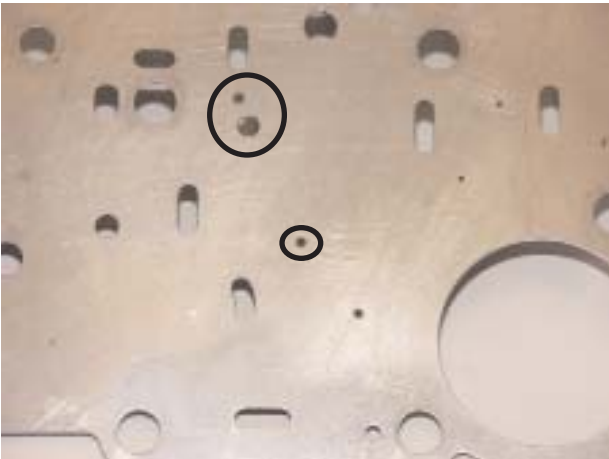
Type 2 Valve Body Plate Must Match Case
