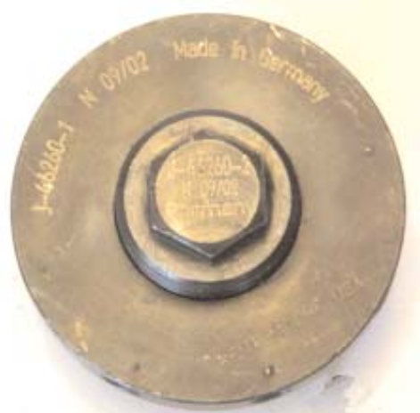
Late Model 3-4 Accumulator Cover Removal Tool Kent Moore Tool # J-46260-1
