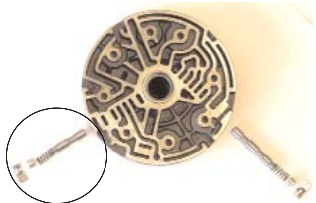
Type 2 Center Support with Valves Out. Reverse Inhibit Valve not used in All Models
