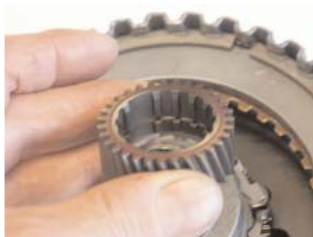
Install Overdrive Sun Gear with Lube Slot Short Offset Down Toward Drum
