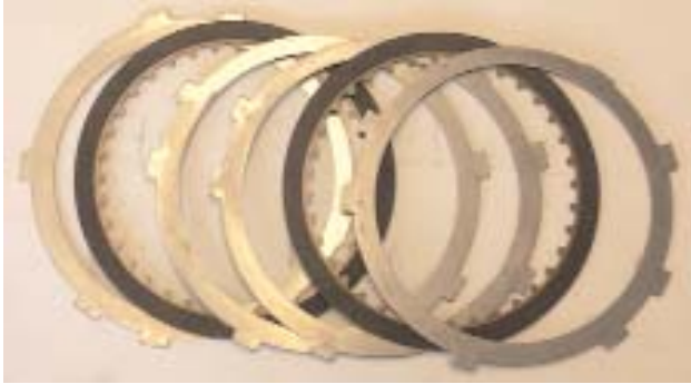
Overdrive Clutch Stack Up
