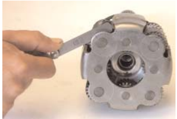
Checking Planet Pinion Endplay Clearance Should be .005 - .035
