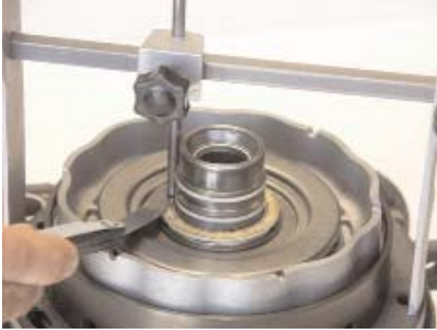
Checking Rear Unit Endplay. Clearance should be .014 - .031 Washer is Selective
