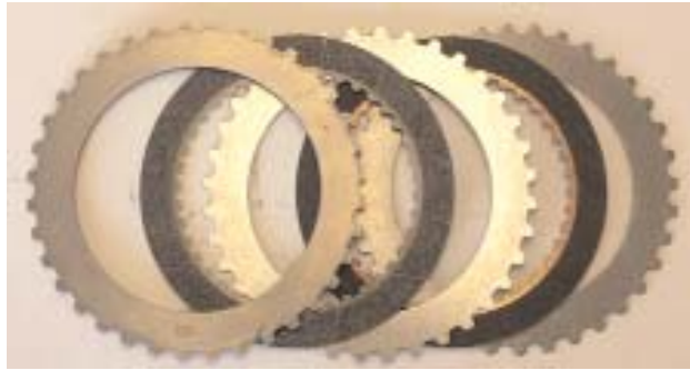
Overrun Clutch Stack Up with Two Frictions (Goes with Picture on Page 4)
