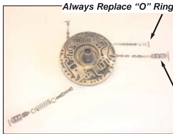
4 Valve Pump (PWM TCC)
