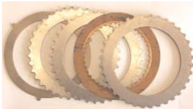
Overrun Clutch Stack Up with Wave Plate
