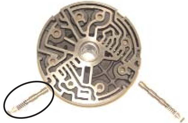
Type 1 Support with Valves Out. Reverse Inhibit Valve Not used in All Models
