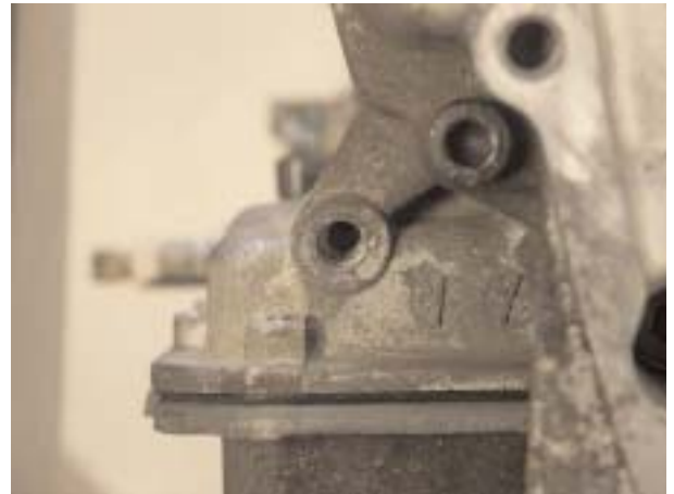
Drilled Case to Check Servo Release Pressure
