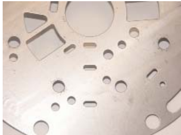
Center Support Spacer Plate without Reverse Inhibit Valve
