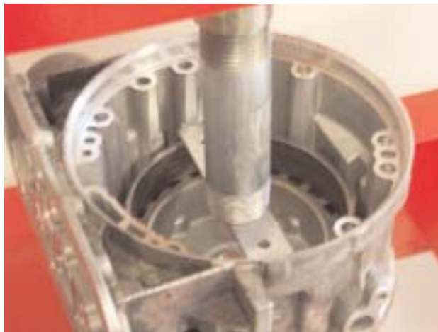
Removing Overdrive Piston return Spring using Tool made from A404 Reverse Band
