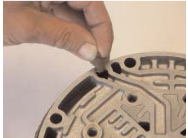
Lube Orifice Location in Overdrive Housing
