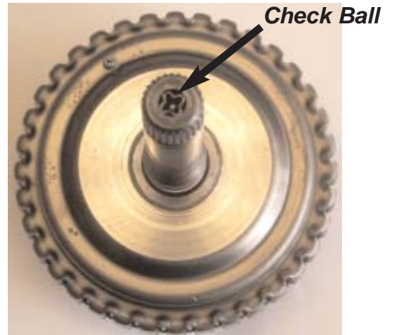
On/Off Torque Converter Clutch has a Check Ball in the End of the Input Shaft. PWM Torque Converter Clutch Does Not
