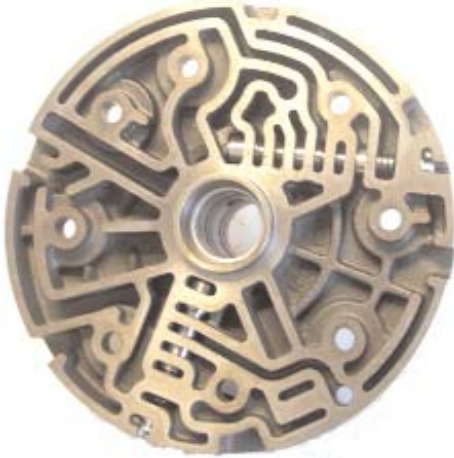
Type 1 Center Support uses Roll Pins to Retain Valve End Plugs
