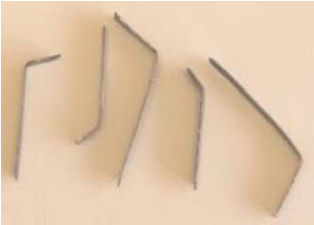
Tools to Disassemble 3rd Clutch Drum made from .010 - .012 Spring Steel 3/16" Wide
