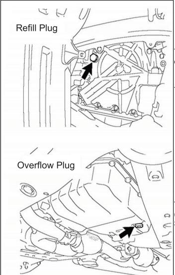
The fluid level must be set at a temperature range of 40°C (104°F) to 45°C (113°F).
