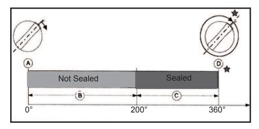
The fuel cap may stay within the (C) range, since it is a large range. A leak is unlikely to occur, even if the fuel cap was not closed completely (until clicking sound is heard (D)).
